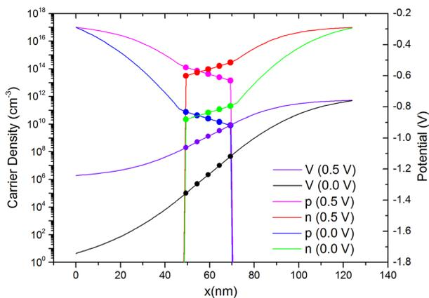
FIG. 4. Carrier densities and electrostatic potential in a device with 5 QD layers (represented by dots on the plot) at equilibrium and with an applied voltage of 0.5 V.
