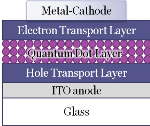
FIG. 1. Schematic device structure for a quantum dot light emitting diode.
