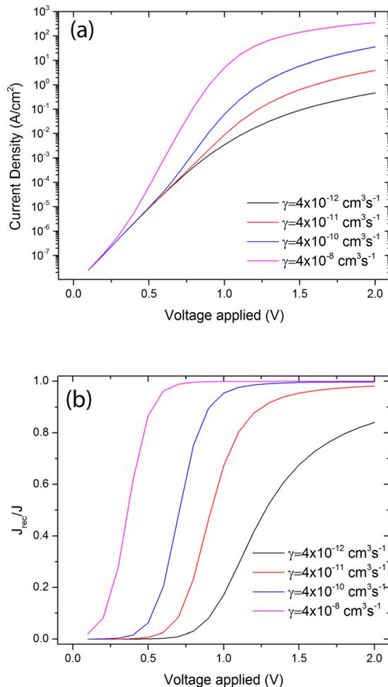
FIG. 7. (a) Current density vs applied voltage and (b) ratio of recombination current to total current ( $J_{\text{rec}}/J$ ) for various radiative recombination coefficients ( $\gamma$ ).
