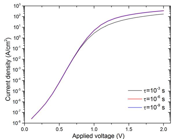
FIG. 6. Current density vs applied voltage for different assumed values of the carrier capture coefficients ( $\tau$ ).
