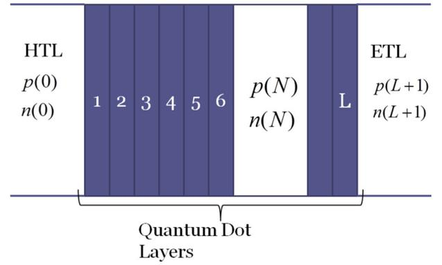
FIG. 3. Discretization scheme for QD-LED focusing on the QD layers.
