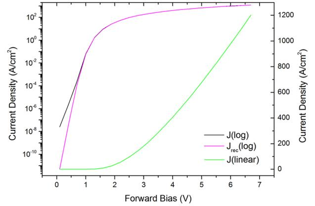
FIG. 5. Total device current density (log and linear) plots with increasing forward bias. The recombination current density is also plotted.
