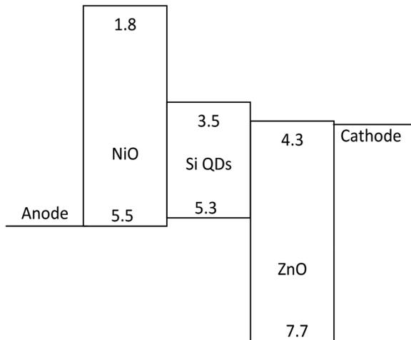
FIG. 2. Flat band diagram for a sample device which consists of Si quantum dots, ZnO as the electron transport layer, NiO as the hole transport layer, and ohmic contacts to both anode and cathode. The horizontal lines at ends signify the metal Fermi energies for anode and cathode. Energies are in eV with respect to the vacuum level.
